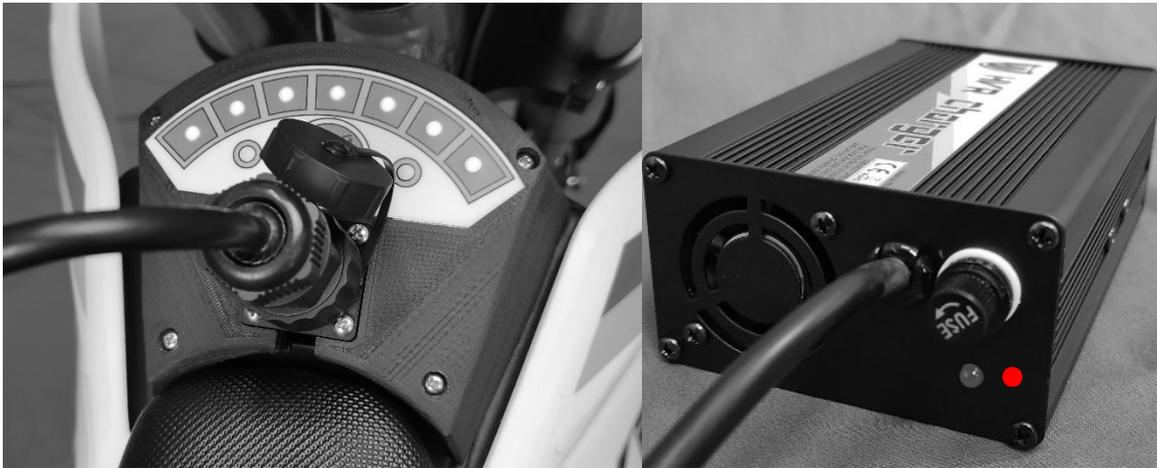
▷ The flashing green LED on the motorcycle shows the current SOC.
