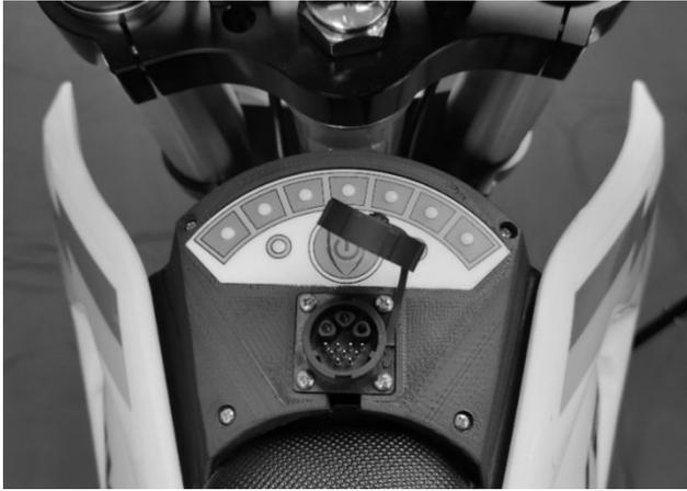
▷ Connect the charger's charging plug to the charging port of the motorcycle (bayonet closure), charging now starts automatically and the LED on the HVR charger lights up red.
