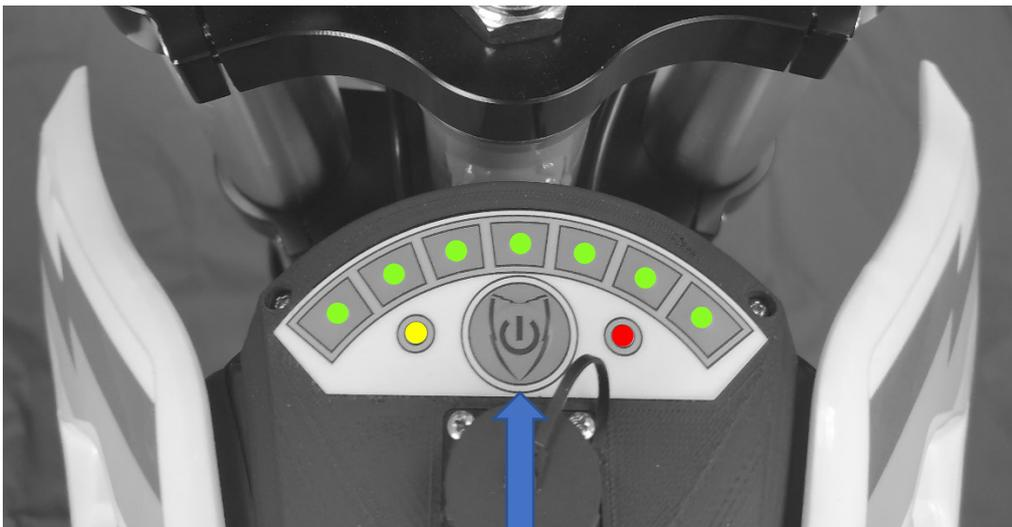
The on/off switch is in the middle of the display.
